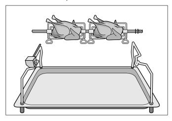
5 Place the rotisserie spit on the supports. Latch the square shaft into the drive section.
