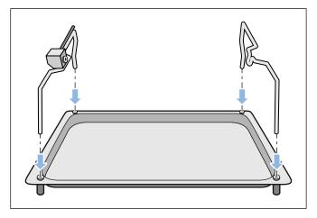
2 Plug the right retaining clip onto the rotisserie spit and screw it in firmly.
