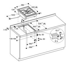
A: When installing with appliance cover, take the deeper cut-out into consideration (observe separate planning notes) B:  $3.5^{\pm 3}$  measurements in mm
