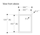
A: When installing with appliance cover, take the deeper cut-out into consideration (observe separate planning notes) measurements in mm
