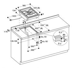
A: When installing with appliance cover, take the deeper cut-out into consideration (observe separate planning notes) B:  $3.5^{\pm 3}$  measurements in mm
