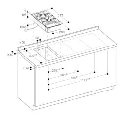
Minimum distance from the appliance cut-out to the side wall 150 mm.
