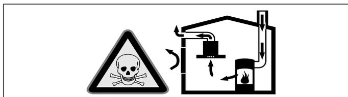
Non-room-sealed heat-producing appliances (e.g. gas-, oil-, wood- or coal-powered heaters, continuous flow heaters or water heaters) draw in combustion air from the room in which they are installed and discharge the exhaust gases into the open through an exhaust gas system (e.g. a chimney).
