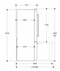
${\bf A}:$  Front is adjustable from 1830 to 1847, with front levelling feet fully extended  ${\bf B}:$  With handle
