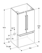
A: Front is adjustable from 1830 to 1847, with front levelling feet fully extended. B: Add 25 mm for fixed spacers on back C: Water connection position
