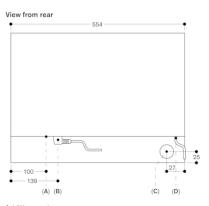
A: LAN connection B: Electric terminal box C: Water outlet D: Cold water inlet
