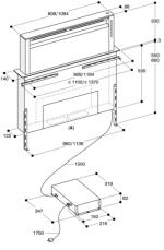
A: Flexible connection of the hood at the front, the back, or at the bott
