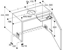
\* for upper cabinets measuring 90 cm, the AA 210 491 installation set is required in addition
