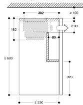
measurements in mm
